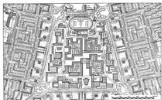
FIG. 48. The Town Centre of the Theoretical New Town. With an area of some 45 acres, it includes both a stadium and a Technical College. The Ambulance and Fire Stations, however, are placed outside the Centre itself within the Industrial Area, from which are likely to separate many of the most serious calls on their services. It will be seen that the design of the Centre follows the "inner-inner ring road" principle, the main shopping core being limited to pedestrian usage for car parks.
