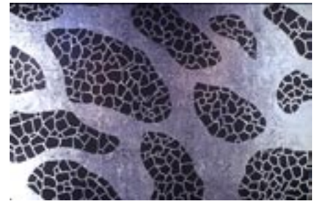
Screen-printed galvanised steel. The metal background will oxidise, go grey and lose its sheen. Clear-lacquer will slow this down, but not for ever.
